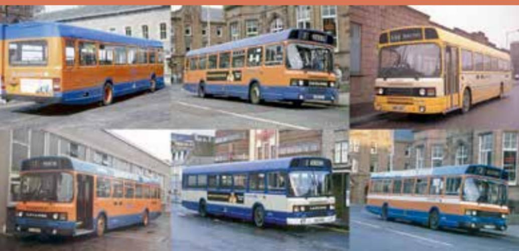
The four buses from Northern Scottish were 10-6m long with single door. Two of them had no roof pod (SN4 GS07V/KRS541V, SN5 GS08V/KRS542V/PIL2755) and the other two carried short roof pods (SN10 MSO 9W, SN11 MSO 11W).
